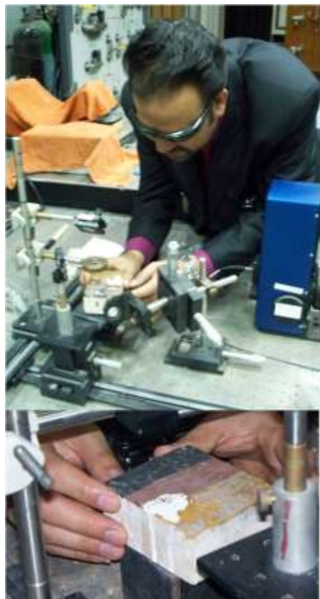
Fig. (5): The wall painting models during laser cleaning,( notice the difficulty of gypsum incrustation removing).
