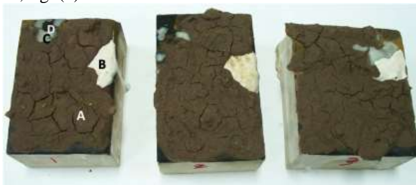
Fig. (1): the wall painting models after adding the deterioration aspects: a) mixed mud with gypsum, b) gypsum, c) wax and d) soot.
