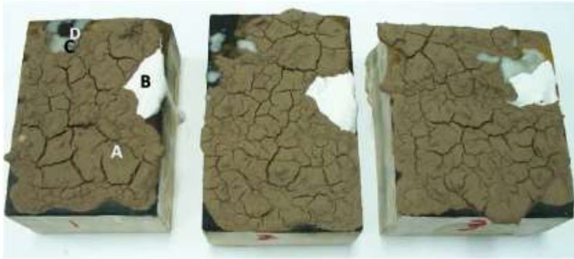
Fig.(2): The wall painting models after the artificial ageing cycles: a) mixed mud with gypsum, b) gypsum, c) wax and d) soot.
